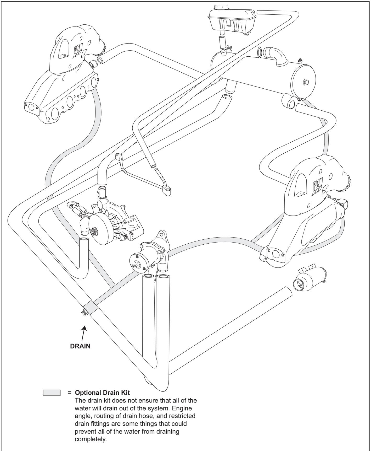
**Figure 15-4** Water Drain kit - Optional (6.0L)
