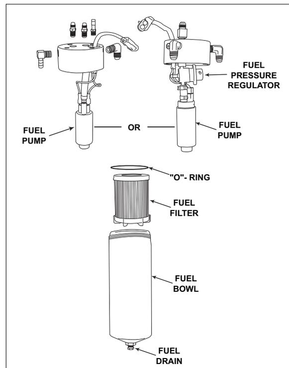
**Figure 11-13** Fuel Control Cell (FCC) - Screw-on Canister (Typical)
