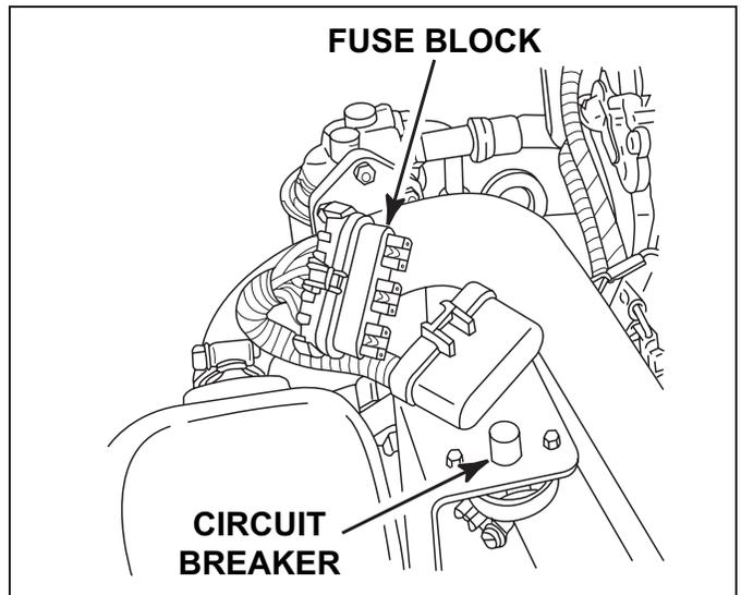
**Figure 11-5** Typical Electrical System Circuit Breaker and Fuses
