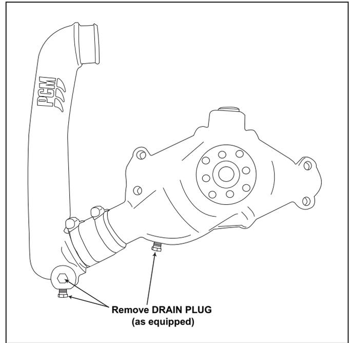
**Figure 13-2** Draining Engine Circulating Pump (5.0/5.7L)
