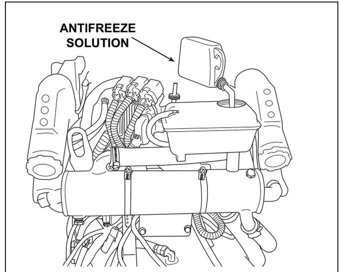
**Figure 11-10** Filling F.W.C. System (6.0L)
