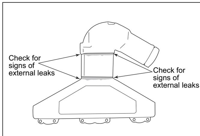
**Figure 5-2A** Water Leaks
