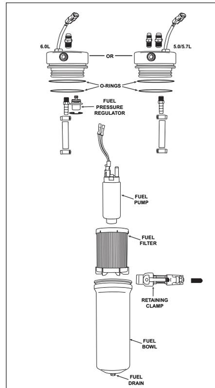
**Figure 11-14** Fuel Control Cell (FCC) - Clamp-on Canister (Typical)
