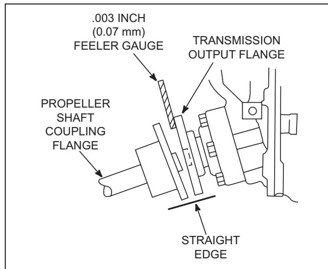
**Figure 11-26** Angular Alignment
