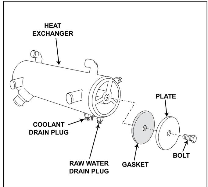
**Figure 11-11** Heat Exchanger and End Plate Removal (Typical)
