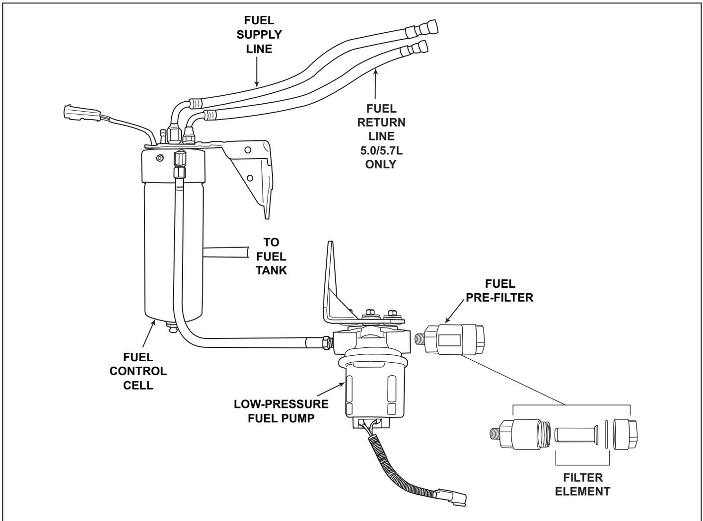
**Figure 11-12** Fuel Control Cell (FCC) Fuel System (Typical)
