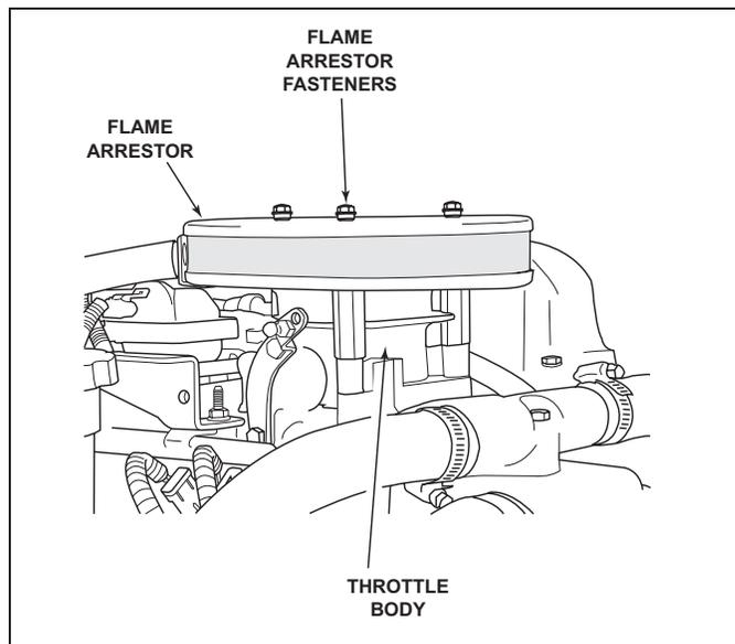
Figure 11-15 Flame Arrestor - 5.7L (Typical)
