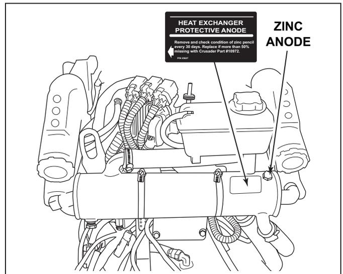
**Figure 11-6** Zinc Anode Location F.W.C. Heat Exchanger (6.0L)
