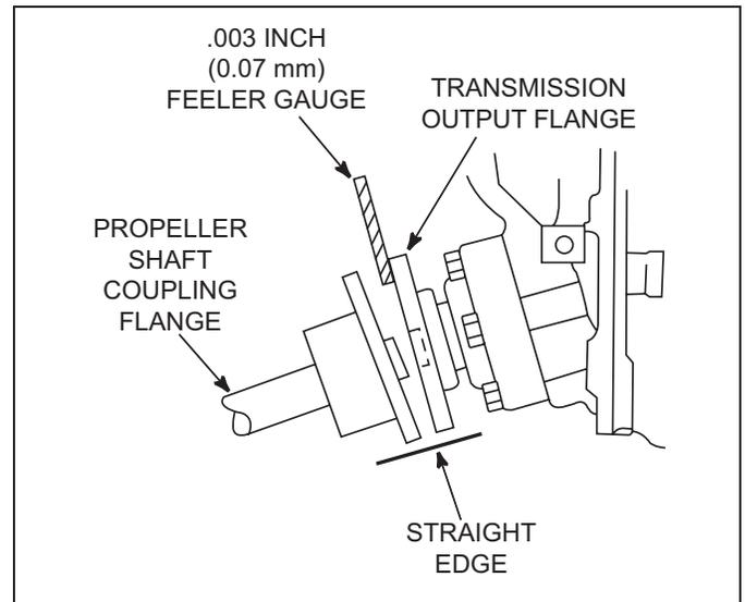
**Figure 11-30** Angular Alignment
