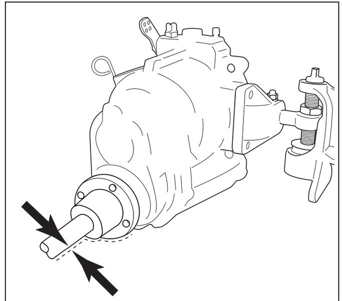
**Figure 11-23** Angular Alignment
