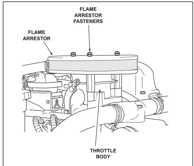
Figure 11-14 Flame Arrestor - 5.7L (Typical)
