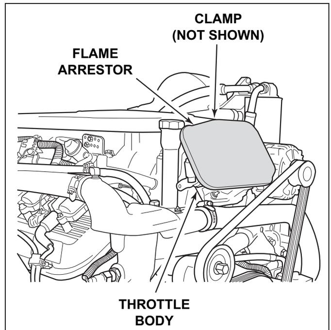
Figure 11-15 Flame Arrestor - 8.1L (Typical)
