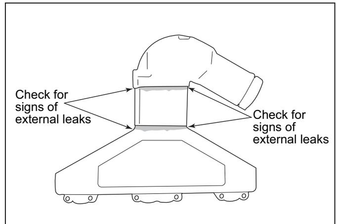
**Figure 5-2A** Water Leaks
