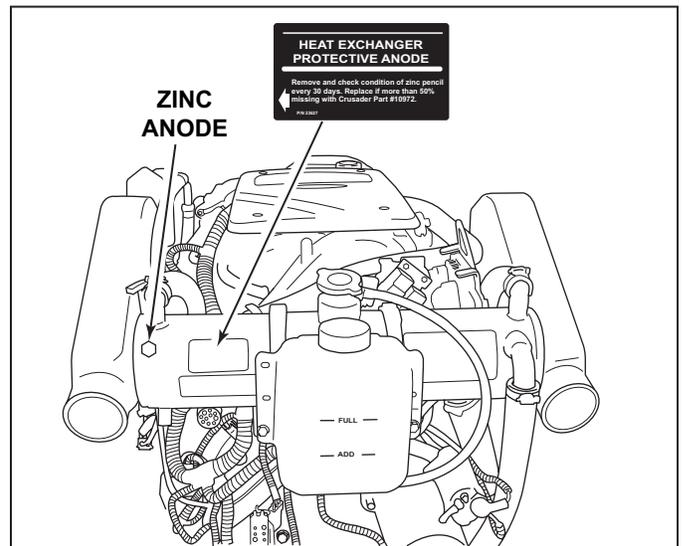
**Figure 11-6** Zinc Anode Location F.W.C. Heat Exchanger (8.1L)
