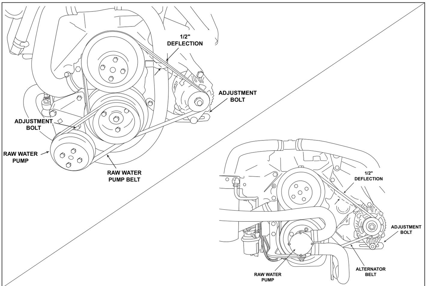
Figure 11-18 Drive Belt Location and Adjustment (5.0L / 5.7L)
